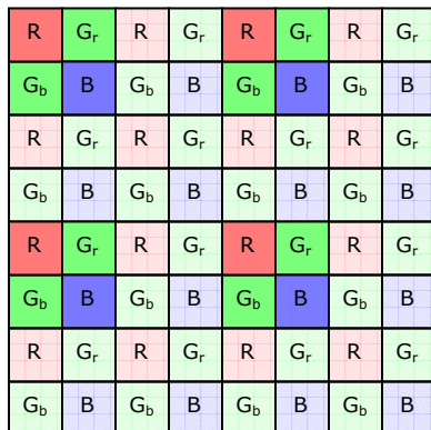
Figure 4: Alternate method for creating a video stream with a Bayer CFA sensor which employs skipping every other RGGB group of pixels
