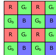
Figure 1: Typical Bayer CFA schematic showing the arrangement of red, green, and blue pixels.
